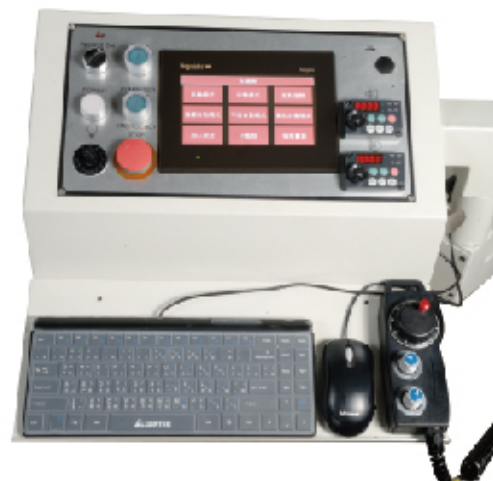
• HMI operation panel and hand-wheel.
